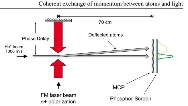
**Figure 3.** A top view showing the horizontal atomic beam subject to the transverse laser beams as it enters the interaction region. The plot at the end is a trace of the atomic flux across the middle of the image. Atoms are deflected by the ARP force, and their velocity distribution is broadened by the width of the longitudinal velocity distribution and by different numbers of spontaneous emission events.
